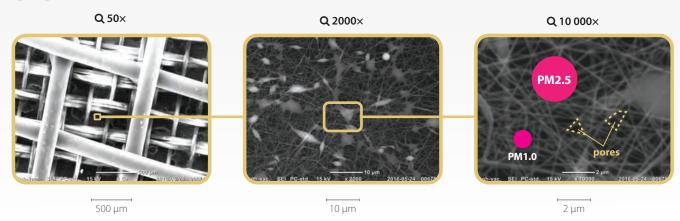
Nanofiber membrane creates a mechanical barrier which prevents the penetration of dangerous particles without using any dangerous chemical substances.
